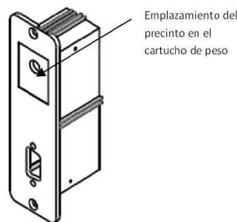
Figure 11. Initial seal position
